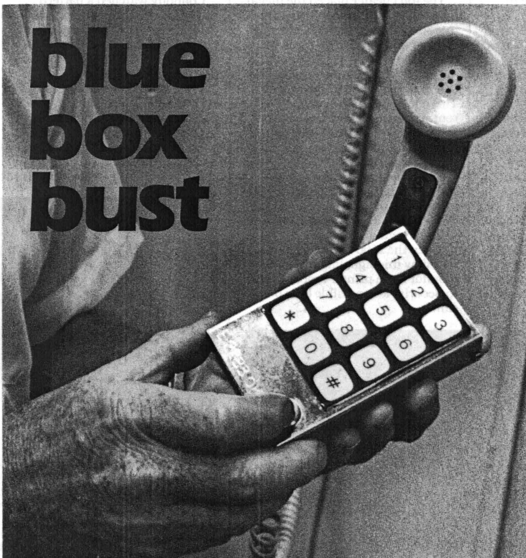
The infamous "blue box," when held to a telephone mouthpiece, can send signals that fool our switching equipment, letting cheaters use our lines toll-free.
